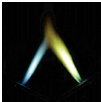
Figure 1. Schematic of the FSP setup using two separate nozzles. The image shows two flames producing Pt/Ba/Al 2 O 3 (blue flame (left): Al; yellow-greenish flame (right): Pt and Ba).
